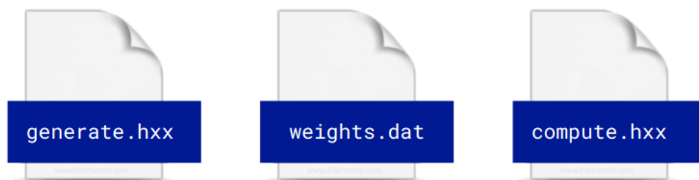
Fig 5: To integrate a custom operator, the user has to supply the compute function in an additional header file which will be included in the generated inference code.
